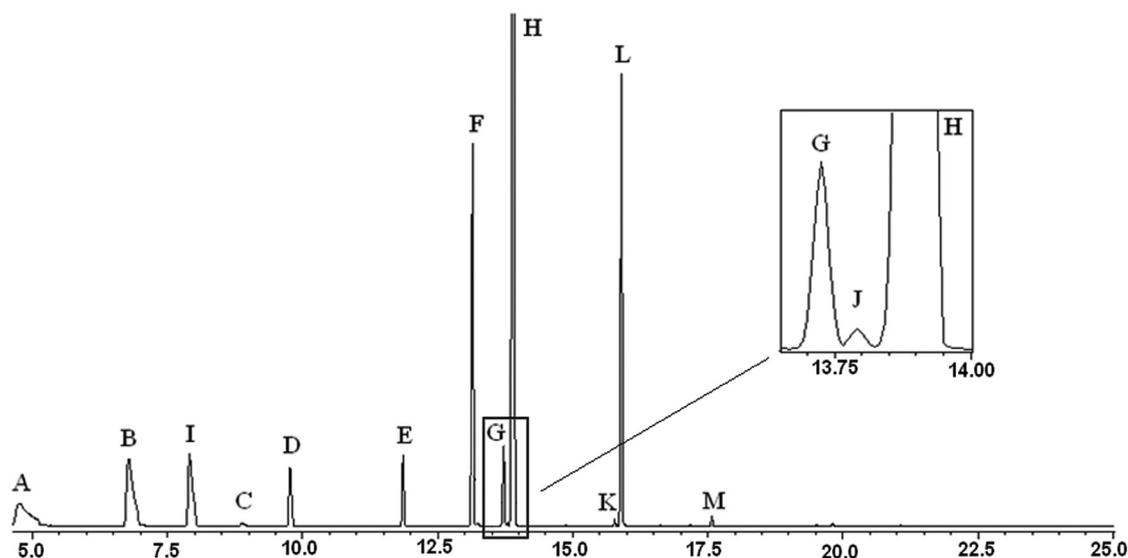
**Figure 2.** Gas chromatogram of a metathoracic gland extract of a *P. macunaima* adult female 10 days-old. Compounds: A: (*E*)-2-hexenal, B: (*E*)-4-oxo-2-hexenal, C: (*E*)-2-octenal, D: undecane, E: dodecane, F: (*E*)-2-decenal, G: 1-tridecene, H: tridecane, I: (*E*)-2-hexenyl acetate, J: (*E,Z*)-2,4-decadienal, K: tetradecane, L: (*E*)-2-decenyl acetate, M: pentadecane.
