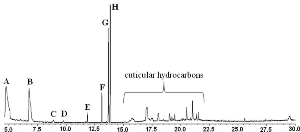
**Figure 1.** Gas chromatogram of exuviae extract from a fifth-instar *P. macunaima* nymph. Compounds: A: (*E*)-2-hexenal, B: (*E*)-4-oxo-2-hexenal, C: (*E*)-2-octenal, D: undecane, E: dodecane, F: (*E*)-2-decenal, G: 1-tridecene, H: tridecane.
