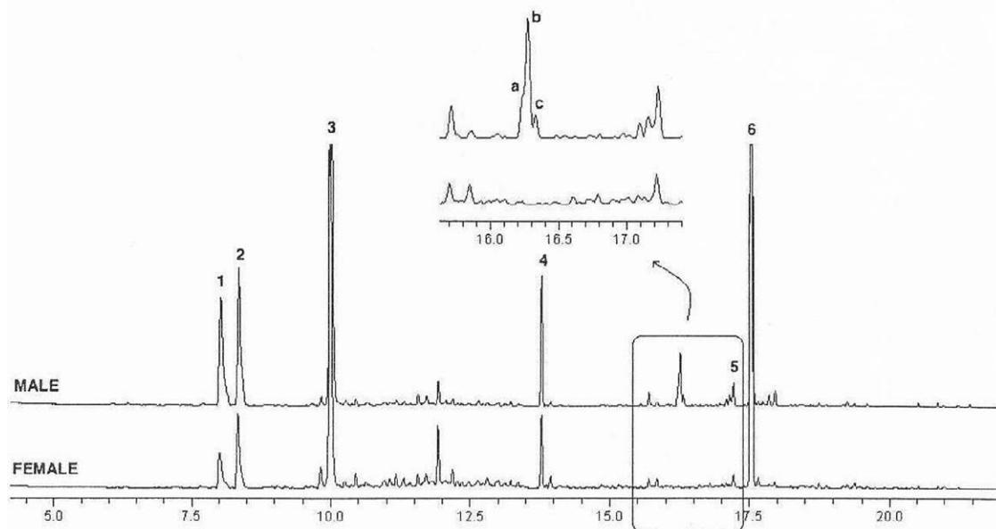
Fig. 1. Comparison of the 96-h aeration extract chromatograms of males and females of *Uломoides dermestoides*. 1: methyl-1,4-benzoquinone; 2: limonene; 3: ethyl-1,4-benzoquinone; 4: 1-tridecene; 5: pentadecadiene; 6: 1-pentadecene; a-c: male-specific compounds.
